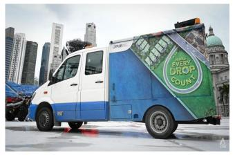
The PUB water wagon is equipped with a 1,000L tank to provide potable water during water disruptions.
