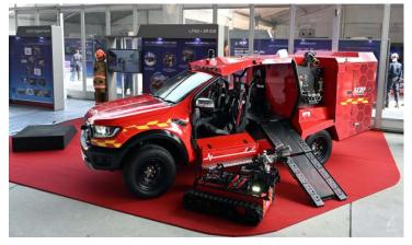
The 6th Generation Light Fire Attack Vehicle (LF6G) is equipped with the second generation of the Red Rhino Robot (3R 2.0) to allow firefighters to operate from a safe distance during fire incidents.
